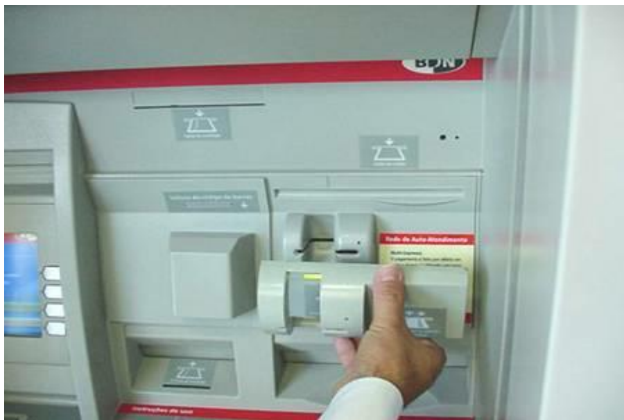
Equipment being installed on front of existing bank card slot.
